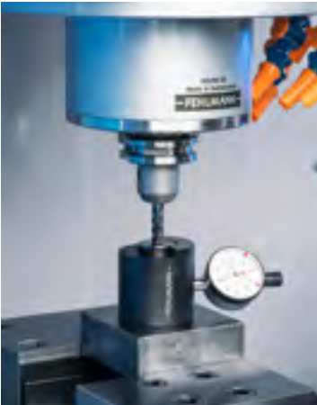
The TOP package includes: Tool setter for manually plotting the Z-axis zero point on a resting spindle.
