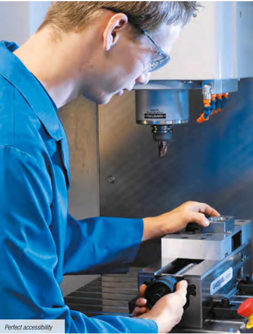
Full flexibility with the TOP functions Drill by hand or start drilling cycles without writing a program. If the end stop is set, or the drilling cycle is defined, the position can be approached by hand, directly in the drilling cycle or using the MDI function – lightning fast and precise.
