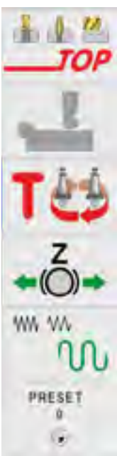
Full flexibility with the TOP functions Drill by hand or start drilling cycles without writing a program. If the end stop is set, or the drilling cycle is defined, the position can be approached by hand, directly in the drilling cycle or using the MDI function – lightning fast and precise.
