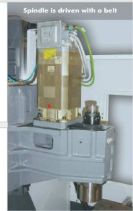
For VX6 / VX8 / VX10 / VX12 Belt Drive For VX4 Spindle Directly Coupled to Motor
